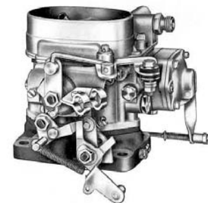
Type 32 PAITA (Downdraught Compound Carburetor)
